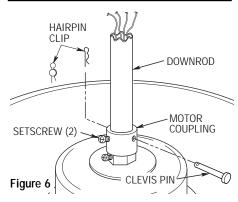
□ **10.** Tighten the setscrews (Figure 6) securely while pulling up on the downrod.
